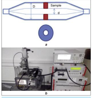
Fig. 2. TEM cell equipment of ICPE-CA: a – operating principle; b – photo of apparatus of the National Institute for R&D in Electrical Engineering – ICPE-CA, Romania
